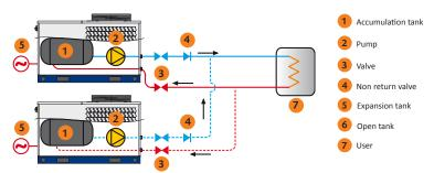
Expansion tanks are required for all closed circuit installations. When multiple chillers are installed in parallel, the expansion tanks must be automatic.
