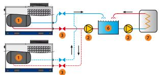
Expansion tanks are not required for open circuit installations. Open circuits also typically use an external pump, so the internal pump may not be required.
