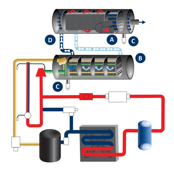
hot, wet compressed air enters the shell of the airto-air heat exchanger. Air is cooled as it circulates around the aluminum finned copper tubes that contain cool air from the air-to-refrigerant heat exchanger
