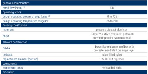
inlet & outlet connections (NPT)
