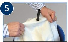
Insert the second filter (needle-felt bag with black inlet tube) and rest it on top of the retainers.
