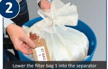
body, settling it down gently, and ensuring it is in contact with the side wall.
