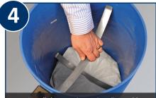
Install the securing spring clips at 90 degrees directly in contact with the filter bags to prevent floatation.
