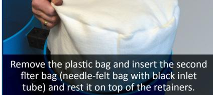
Remove the plastic bag and insert the second filter bag (needle-felt bag with black inlet tube) and rest it on top of the retainers.
