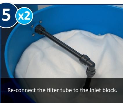
Re-connect the filter tube to the inlet block.
