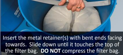
Insert the metal retainer(s) with bent ends facing towards. Slide down until it touches the top of the filter bag. **DO NOT** compress the filter bag.
