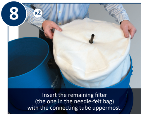
Lower the filter bag 1 into the separator body, settling it down gently, and ensuring it is in contact with the side wall.
