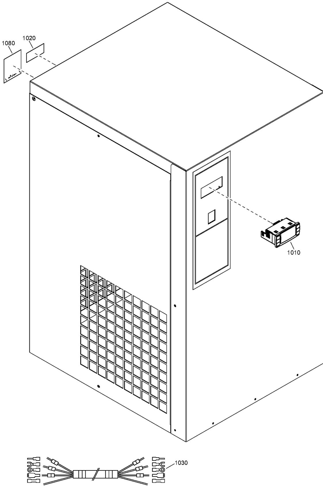
**9 - Electrical components DXR0085N, DXR0105N, DXR0125N, DXR0150N, DXR0185N, DXR0230N - 230V/60Hz - UL-cUL**
