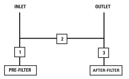
Figure 1.0 - Typical HLX F2-3V Three-Valve Bypass
