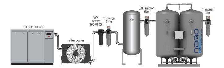
Installation is suggested when the compressed air treated from the dryer is only a part of the total flow rate of the compressor; or when the compressor operates at reduced load and the total consumption equals the compressor flow rate.
