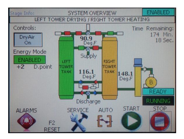
At this portion of time, the right tank is fully depressurized, the blower system will initialize to begin introducing the purge air into the depressurized vessel. After a short amount of time, the heater will be activated and the purge air will be heated to aid in the drying process.
