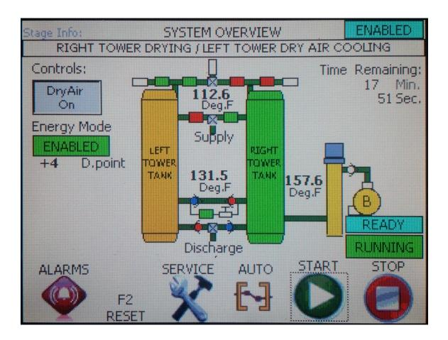
At this portion of the operation, if **DRY AIR COOLING ON** is enabled, the blower will shut down, and the system will use an average of 2% of the compressed air to cool the desiccant bed before the tanks are switched over during the regen process. This prevents dewpoint spikes that can occur during tank switch-over.
