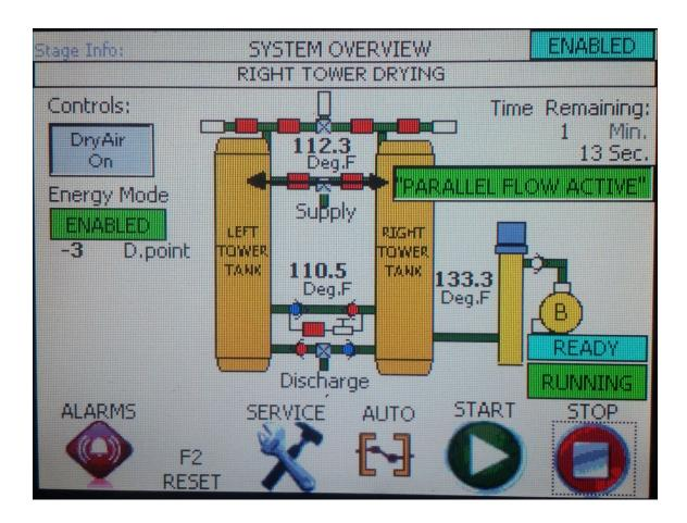
Once the right tank is fully repressurized, this screen will show before the system continues to automatically step throug the drying process.
