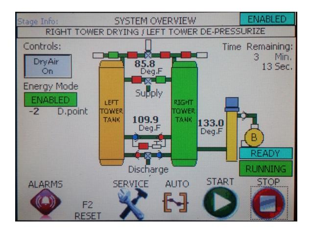
Once the dryer is ready to be put into operation the customer must first pressurize both towers before turning the dryer on. See section 4.7 before operating dryer
