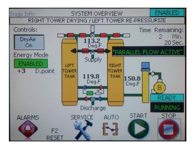
During this stage, the tower will begin to repress the unpressurized tank to plant air psi. Also, at this time, the parallel flow control will show as active. During this process, the purge valves are both shut, and the cool air and the warm air from the previously active tank will mix. This process is activated to prevent dewpoint spikes during tank switchover.
