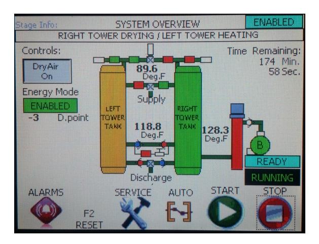
After the left tank is fully depressurized, the blower system will initialize to begin introducing the purge air into the depressurized vessel. After a short amount of time, the heater will be activated and the purge air will be heated to aid in the drying process.
