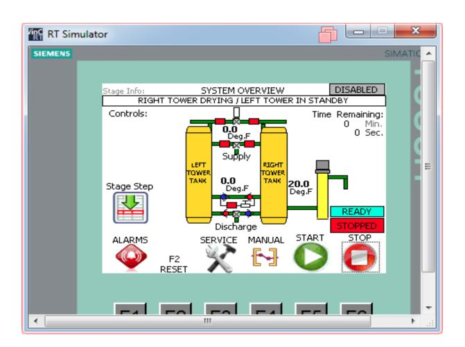
If a dewpoint monitor is installed, and the low dewpoint set point level is reached, the machine will not shut off but will remain in a standby condition. When the dewpoint rises above the high dewpoint set point, the machine will be commanded back to normal operation, and will function until the low dewpoint set point has been met.
