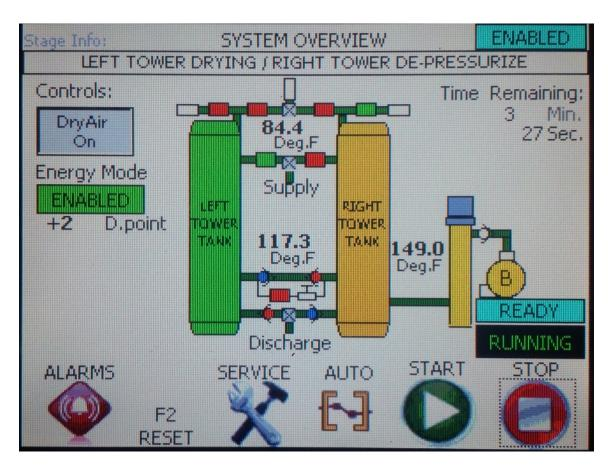
During this process of regen, the left tower will begin the drying process and the right tower will be depressurized. High and Low pressure switches are in place to ensure the system switch-over is initialized on the proper tanks.
