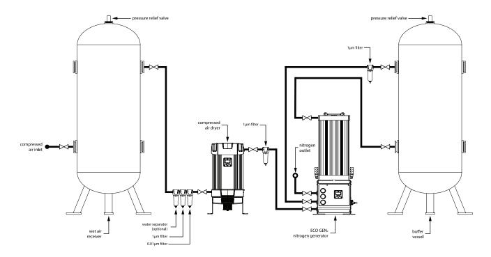
**IMPORTANT**: It is essential that the system into which the generator is installed is fitted with a pressure limiting/relief device. This device should be installed between the compressor and the product.
