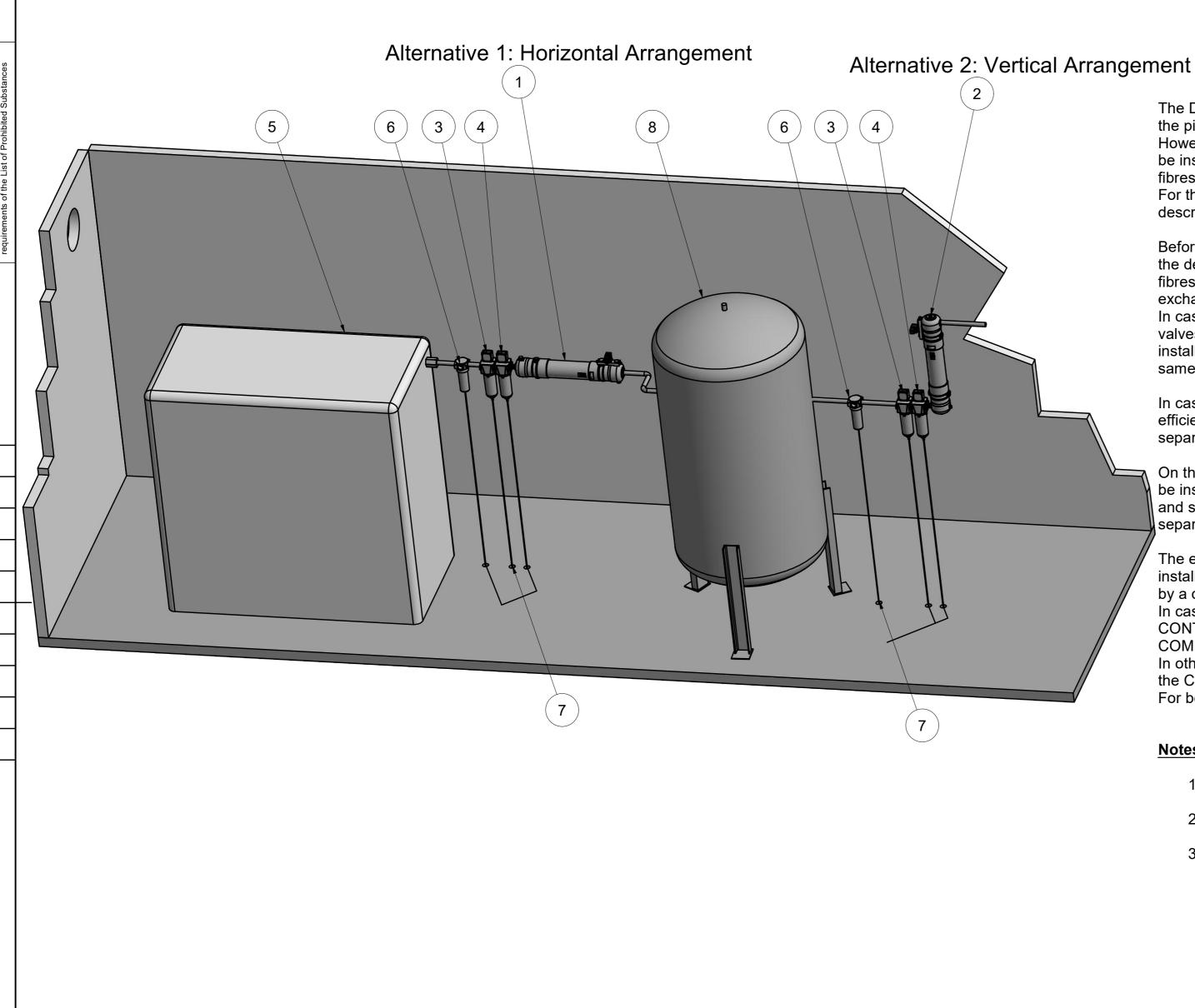
The DHM-DRYER UNIT can be installed HORIZONTALLY (1) or VERTICALLY (2) in the piping network, BEFORE or AFTER the AIR RECEIVER (8).
