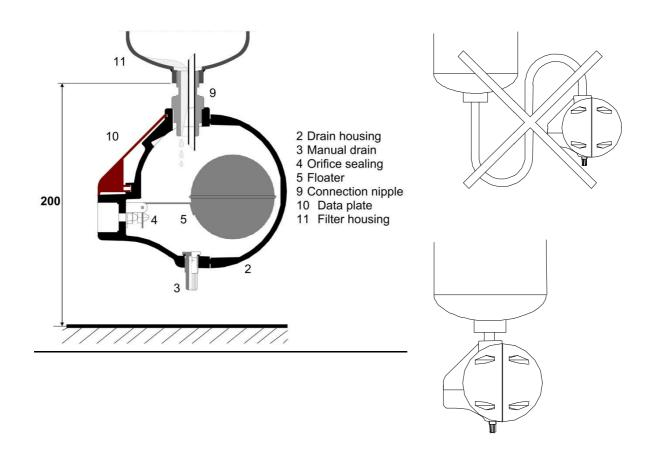
Before connecting the drain, blow compressed air through the piping in order to thoroughly clean out any impurities within it.
