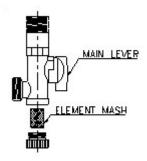
The Y-strainer provided with the condensate drain helps to trap particulate contamination and minimize the potential for leakage at the drain seat. It is necessary to clean the Y-strainer periodically to maintain proper operation of the drain. How often depends on cleanliness of the compressed air pipework and other components in the compressed air stream. All models from RNC 0010 are equipped with a Y-strainer.
