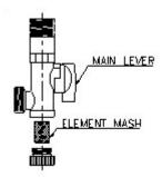
The locally installed strainer on the condensate drain helps to trap dirt. It is necessary to clean the Y-strainer depending on the quantity of the dirt present in the system to ensure proper operation. All our models from RTC 0010 are equipped with this Y-strainer.
