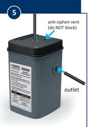
Connect tube into outlet fitting and feed to drain (side). Ensure a steady fall from outlet point to drain with no kinks or tight bends.
