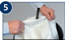
Insert the third filter bag (needle-felt bag with black inlet tube) and rest it on top of the retainers.
