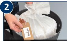
Lower the filter bag 1 into the separator body, settling it down gently, and ensuring it is in contact with the side wall.
