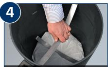
Install the securing spring clips at 90 degrees directly in contact with the filter bags to prevent flotation.
