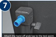
Attach the twist off grab tap to the test point. Attach your outlet hose to the nipple above. Fill unit with water and check for leaks.
