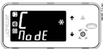
7. Press DOWN: the function for switching from cooling (C) to heating (H) mode (ModE) is shown – for heat pump units only.
