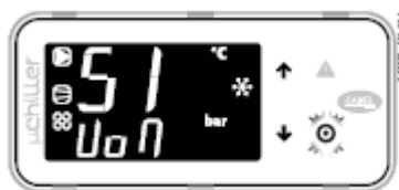
10. Press DOWN: the unit of measure selection (UoM) is shown
