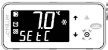
4. Press PRG: the value flashes; press UP/DOWN to change the value; PRG to confirm.
