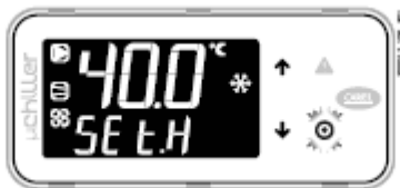
5. Press DOWN: the heating set point (SEtH) is shown - for heat pump units only.
