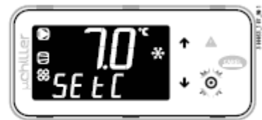
3. Press DOWN: the cooling set point (SEtC) is shown
