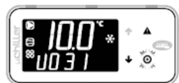
7. Press UP/DOWN to display the other parameters.
