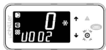
5. Press PRG: the first parameter is shown: U002 (Pump 1 manual control)
