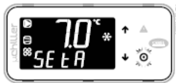
2. Press DOWN for 3 s: the current set point (SEtA) is shown - read-only
