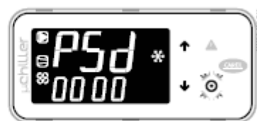
3. Press PRG: the first digit of the password flashes; set the value, press PRG. The second digit now flashes; enter the other digits to complete the password.
