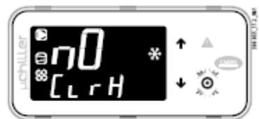
9. Press DOWN: the function to delete the alarm log (ClrH) is shown – Service level only.
