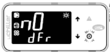
8. Press DOWN: the manual defrost function (dFr) is shown – Service level and reverse-cycle A/W units only.
