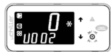
6. Press PRG: the value flashes; press UP/DOWN to change the value; PRG to confirm.
