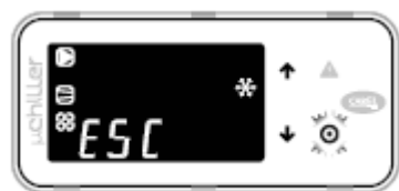
11. After having completed the settings, to exit either: – from the categories press ESC and then PRG; – press PRG for 3 s
