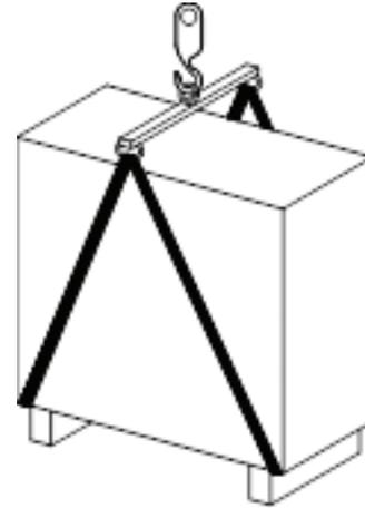
When using straps or ropes to the harness, use a sling bar to ensure that there is no pressure being put on the upper edges of the machines or packaging. Place the straps lifting points as shown in figure.
