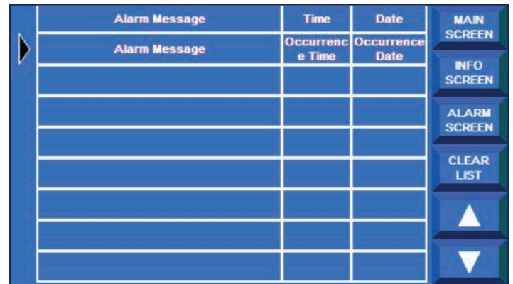
FIGURE 5-5: Alarm Log Screen
