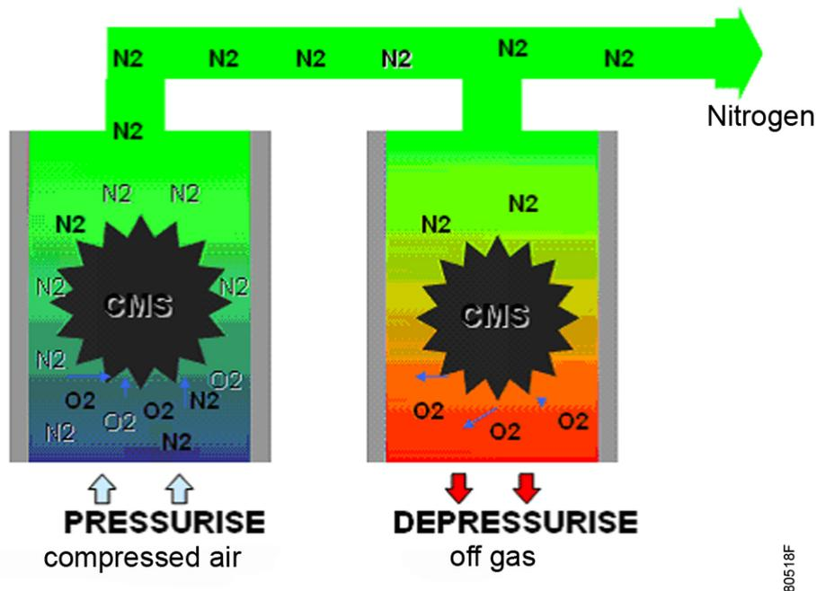
Figure 2: Operating principle of the nitrogen generator
