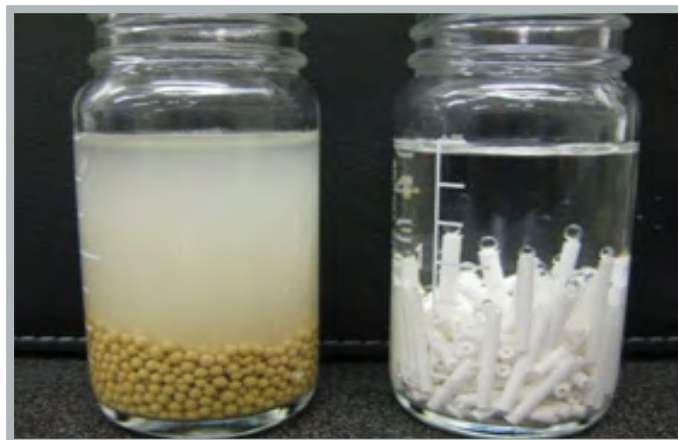
Figure 3 - Granular Desiccant vs. AMT in water
